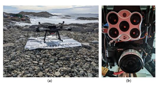
**Figure 3.** UAV and sensors for aerial data collection in ASPA 135. (a) BMR3.9RTK UAV developed by SaiDynamics Australia. (b) MicaSense Altum multispectral (top), and Sony Alpha 5100 high-resolution RGB cameras mounted on the BMR3.9RTK.
