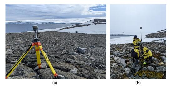
**Figure 5.** Setup to collect GNSS points using a Trimble GNSS kit. (**a**) Base setup using a Trimble R10 antenna placed in a fixed marker with known GNSS coordinates. (**b**) Rover setup using a Trimble R10 antenna for precise GNSS RTK data collection, observing how expeditioners ensured the "no-step" rule over fragile vegetation.
