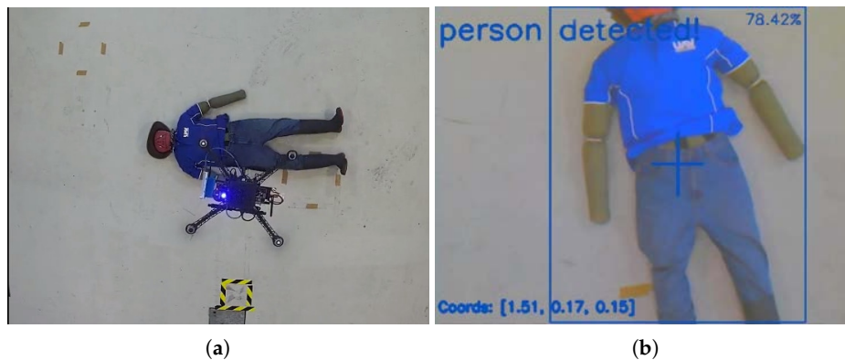
Figure 3. Victim detection trial using the proposed Google MobileNet Single-Shot Detector (SSD) architecture from Chuanqi [48]. Detections with an output score confidence greater than 60% are displayed in the processed frame. (a) Top view of the UAV flying above an adult mannequin. (b) Victim detected with a confidence score of 78.42% after processing raw frames from the HBV-1615 RGB camera.
