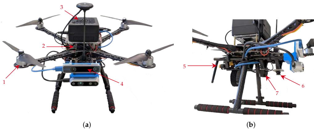
Figure 2. Proposed UAV frame with mounted drivers, companion computer and payload. (a) Front view of the UAV displaying: (1) Holybro S500 frame; (2) Pixhawk 4 ® flight controller; (3) UP 2 companion computer; and (4) Intel ® Realsense ™ T265 tracking camera. (b) Lateral view of the UAV displaying: (5) 433 MHz telemetry radio; (6) HBV-1615 RGB camera; and (7) TFMini Plus range sensor.
