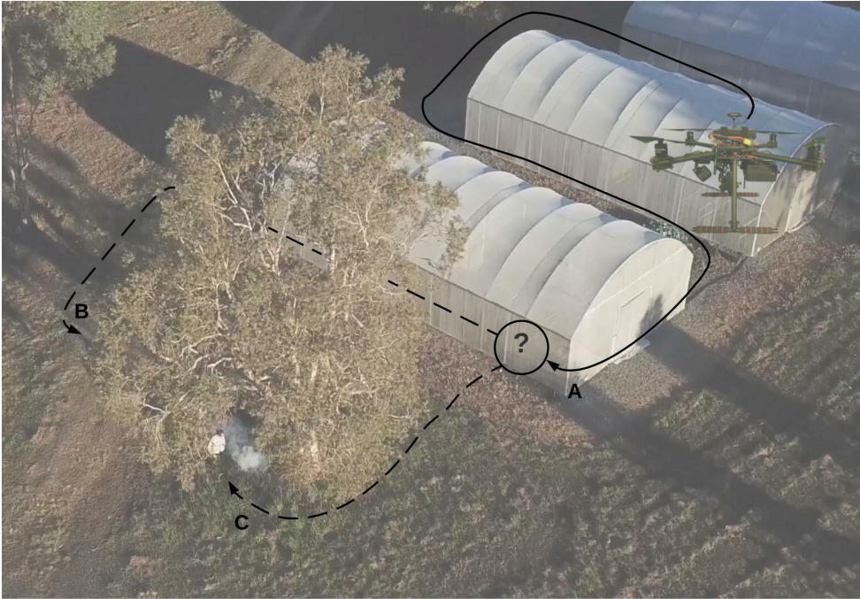
Figure 1.1: Autonomous navigation capabilities onboard small unmanned aerial vehicles (UAVs) for obstacle avoidance, exploration, and object finding in partially observable environments. The path planning strategy (Path A) is subject to mid-flight updates (Paths B or C) as the UAV interacts with the environment and detects potential victims.
