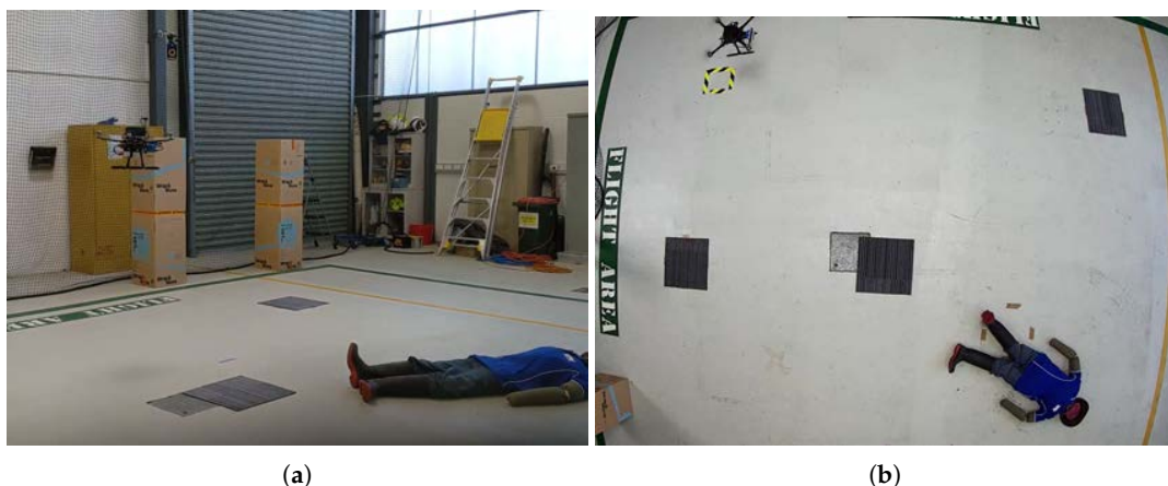
Figure 8. Environment setup for hardware experiments. For safety reasons, an adult mannequin is used as the victim to be detected and column obstacles are replaced with carpet tiles. (a) UAV navigating inside a netted area at the Queensland University of Technology (QUT) Da Vinci Precinct (DVP) hangar. (b) Top view of the setup with the mannequin displayed at the bottom.
