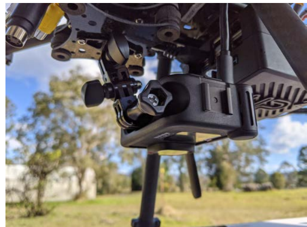
Figure 4. GoPro Hero 9 mounted onto an anti-vibration bracket, pointing to the ground and in parallel to Earth's nadir.
