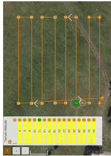
Figure 7. Drafted flight plan in QGroundControl following a lawnmower pattern using the OAK-D camera properties from Table 3.
