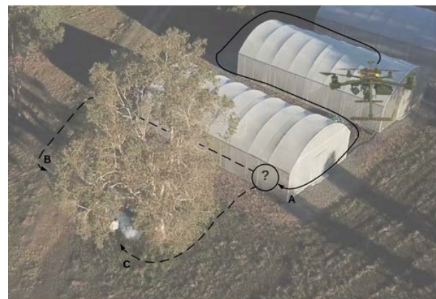
Figure 1. Unmanned aerial vehicle (UAV) navigating in environments under uncertainty and partial observability. A small UAV with autonomous decision-making should be able to plan sequential sets of actions for optimal navigation trajectories, despite limitations from imperfect sensor data.
