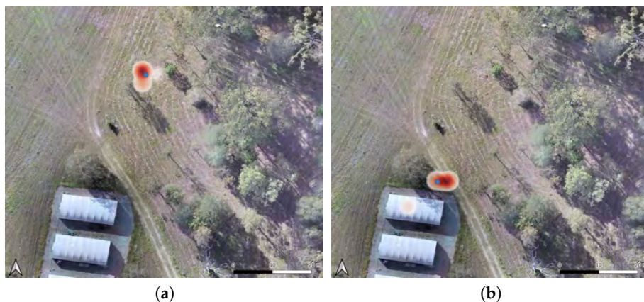
Figure 14. GNSS coordinates' heatmaps of confirmed victim detections by the POMDP-based motion planner in offboard flight mode. (a) First victim location (blue dot) in an open area. (b) Second victim location (blue dot) nearby a tree.
