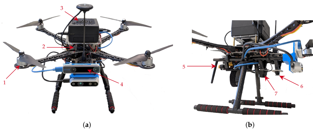
Figure 2. Proposed UAV frame with mounted drivers, companion computer and payload. (a) Front view of the UAV displaying: (1) Holybro S500 frame; (2) Pixhawk 4 ® flight controller; (3) UP 2 companion computer; and (4) Intel® Realsense™ T265 tracking camera. (b) Lateral view of the UAV displaying: (5) 433 MHz telemetry radio; (6) HBV-1615 RGB camera; and (7) TFMMini Plus range sensor.
