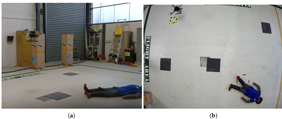
Figure 8. Environment setup for hardware experiments. For safety reasons, an adult mannequin is used as the victim to be detected and column obstacles are replaced with carpet tiles. (a) UAV navigating inside a netted area at the Queensland University of Technology (QUT) Da Vinci Precinct (DVP) hangar. (b) Top view of the setup with the mannequin displayed at the bottom.
